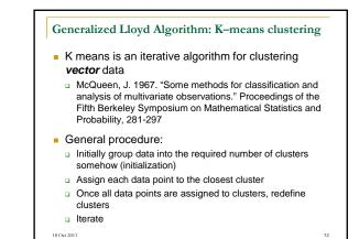
K-means Problem: Given a set of data vectors, find natural clusters Clustering criterion is scatter: distance from the centroid Every cluster has a centroid The centroid represents the cluster Definition: The centroid is the weighted mean of the cluster m<sub>clust</sub> Weight = 1 for basic scheme 18 Oct 201
